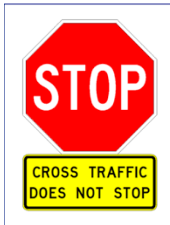
Figure 74 Stop controlled sign with supplemental plaque. Source: TMUTCD
