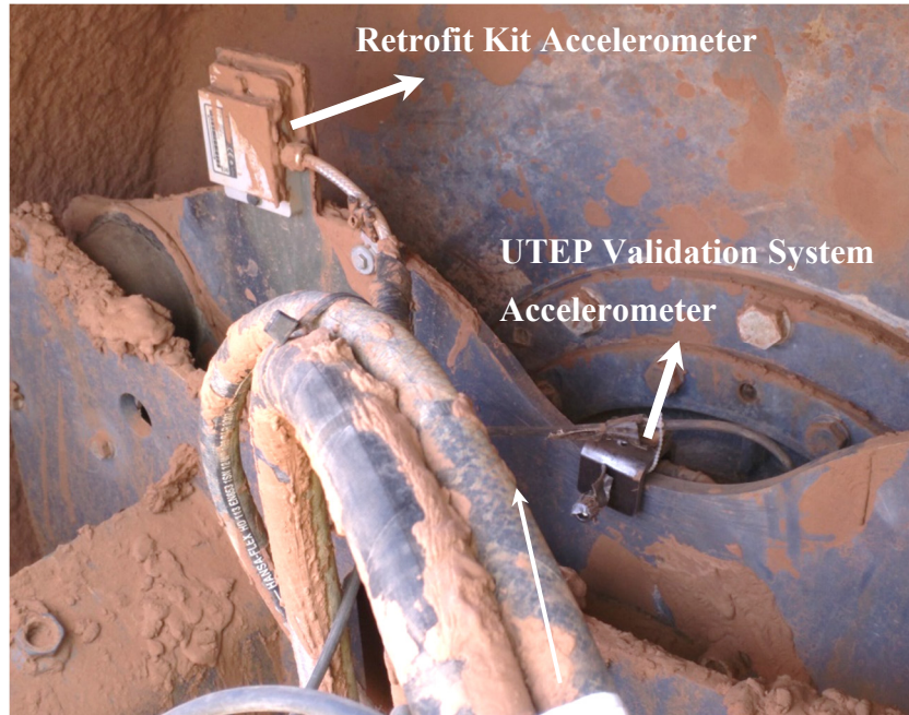
Figure D.2 - Mounted Accelerometers from IC Retrofit Kit and UTEP Validation System.
