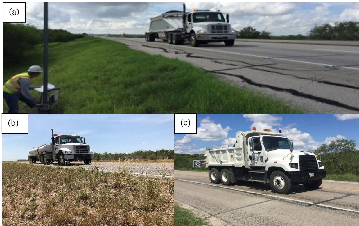
Figure 4.7. Portable WIM Calibration Runs (a) Class 9 Belly Dump (b) Class 9 Water Truck (c) Class 6 Dump Truck
