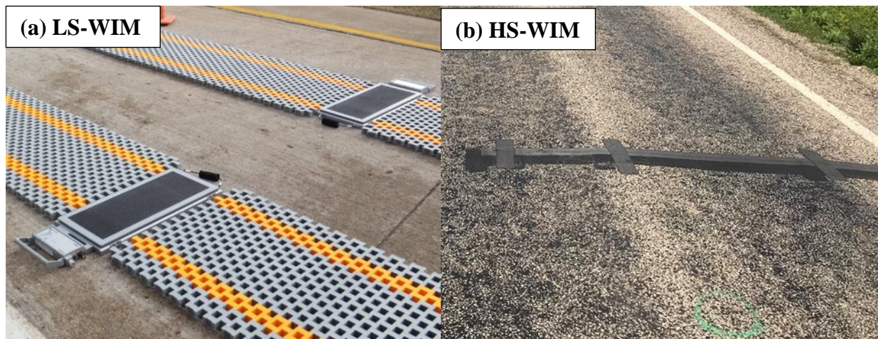
Figure 2.15. (a) Low-Speed Portable WIM and (b) High-Speed Portable WIM. (from Intercomp n.d.)
