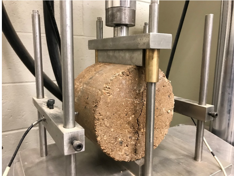
Figure 4-6: Dynamic IDT Test Fixture and Specimen.
