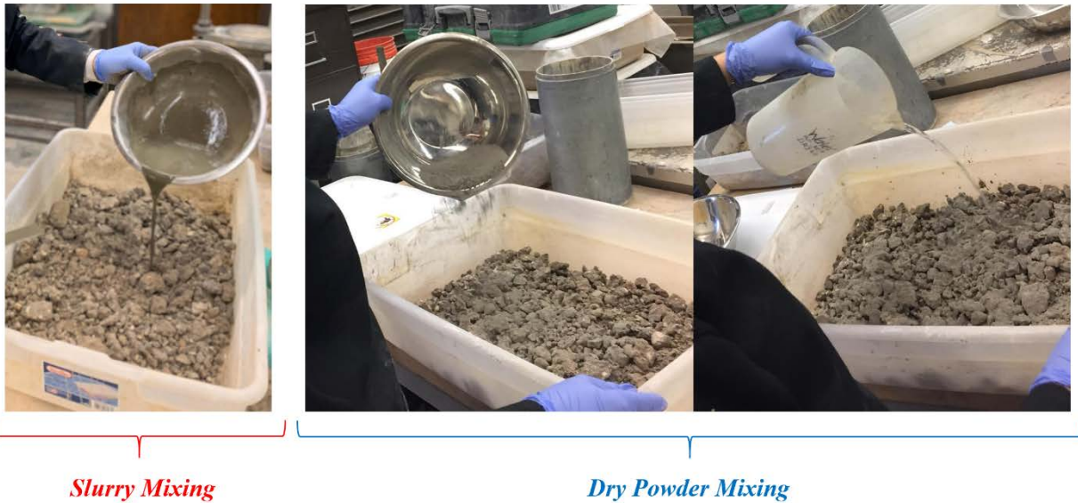
Figure 5-24: Slurry and Dry Powder Mixing Procedures in the Laboratory
