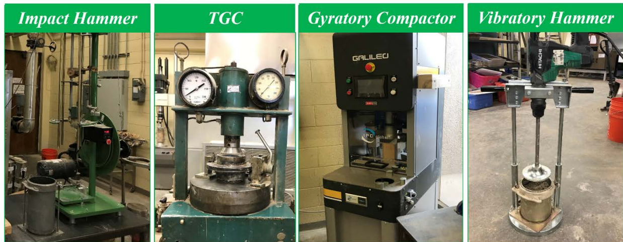
Figure 8-1: Impact Hammer, Texas Gyrotory Compactor (TGC), Gyrotory Compactor, and Vibratory Hammer.
