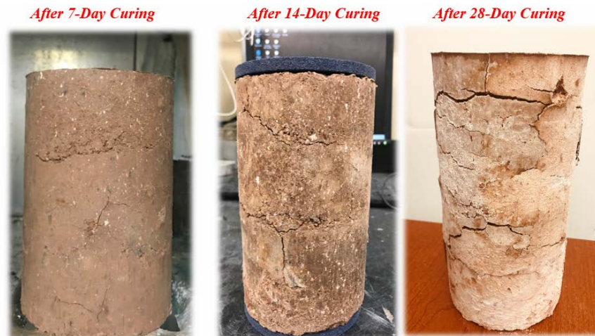
Figure 9-21: Stabilized Clay Soils with 5% Fly Ash and 5% Cement after 7-day, 14-day, and 28-day Curing.
