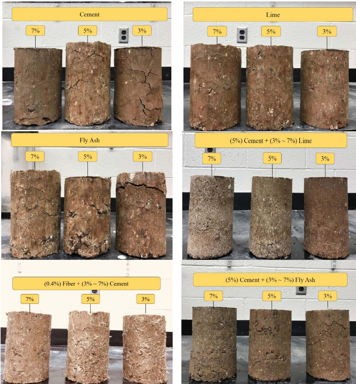
Figure 9-17: Stabilized Clay Soils Sourced from Bryan District after 7 Days of Curing.
