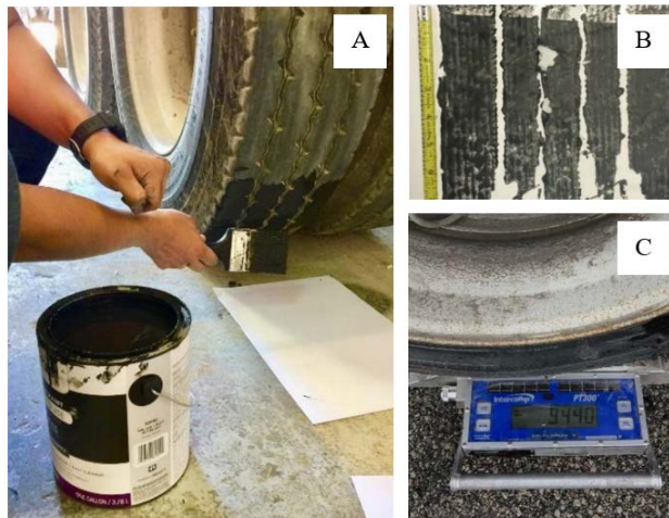
Figure 13-5: Tire Pressure Estimation. A: Painting of Vehicle Tires. B: Print of Painted Tires on Papers. C: Axle Weight Measurements.
