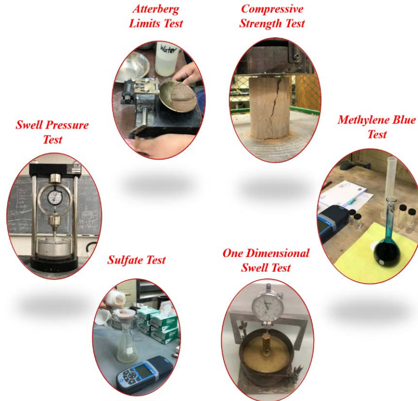
Figure 9-2: Testing Program for Expansive Subgrade Soils.
