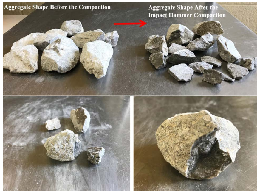
Figure 8-19: Aggregate Breakage during the Impact Hammer Compaction.
