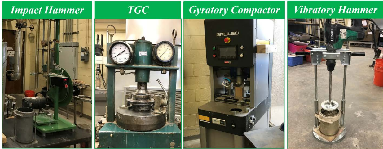
Figure 4-19: Impact Hammer, Texas Gyrotory Compactor (TGC), Gyrotory Compactor, and Vibratory Hammer.
