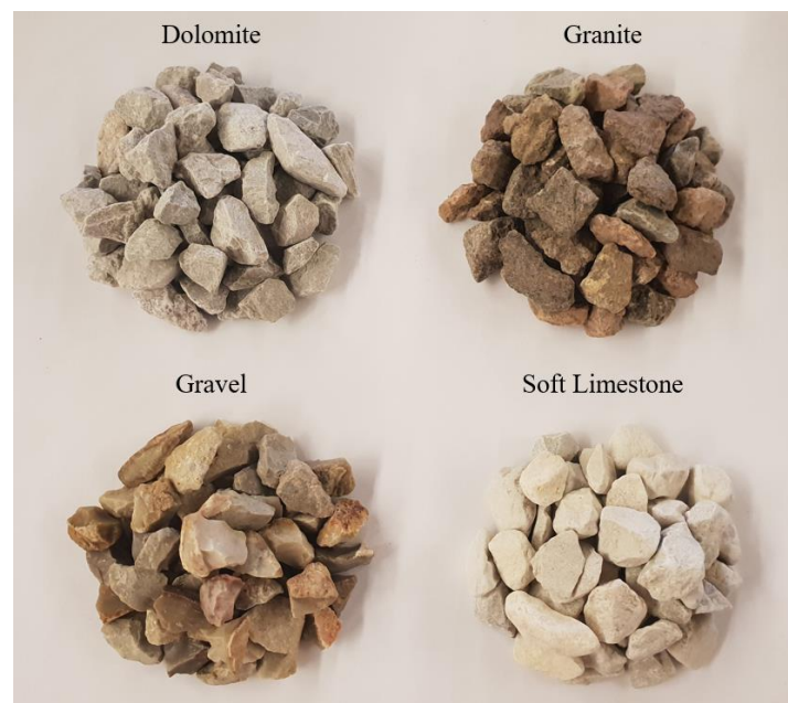
Figure 3.1 - Illustration of Aggregate Shape from 3/8” Sieve Size
