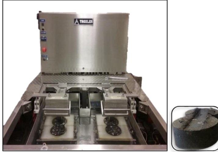
Figure 3.3 - HWT Device and Specimen Setup
