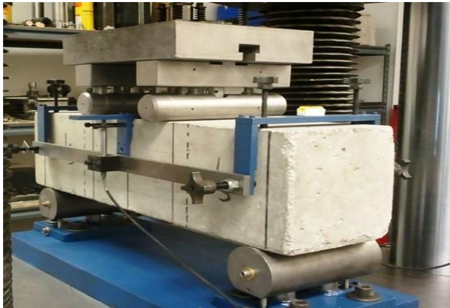
Figure 1.18 – Flexural Beam Test Setup for Modulus of Rupture Testing of Concrete
