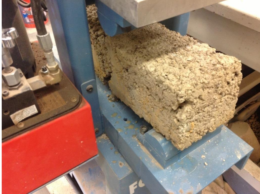
Figure 2.3 – Large Beam Fatigue Test after Failure at UTEP
