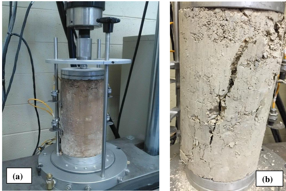
Figure 5.26 – Submaximal Modulus Test (a) Specimen Setup (b) Fractured Specimen
