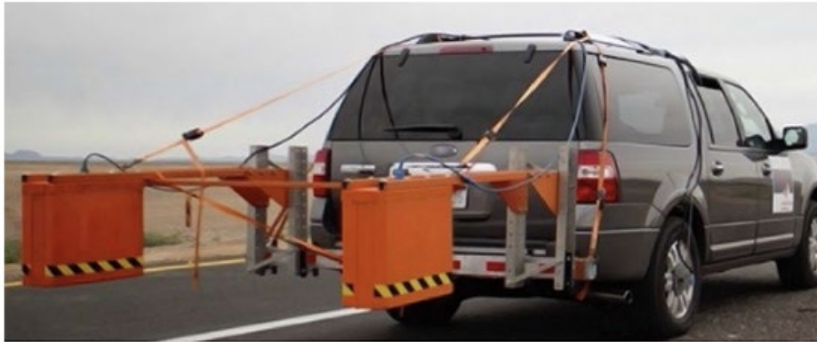
Figure 2: NDOT air-coupled GPR system for bridge deck inspection [1]
