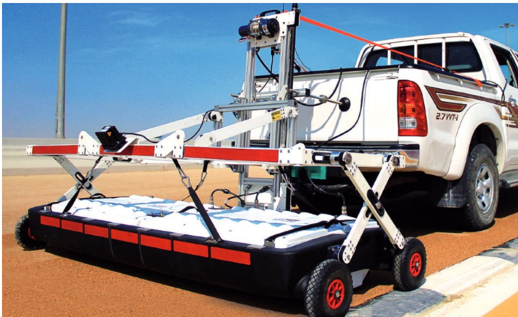
Figure 82. Stream X GPR System Mounted on Survey Vehicle (idsgeoradar.com)
