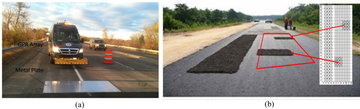
Figure 39: (a) Vehicle mounted with 3D Radar antenna GPR system (b) Pavement containing stripped section[29]
