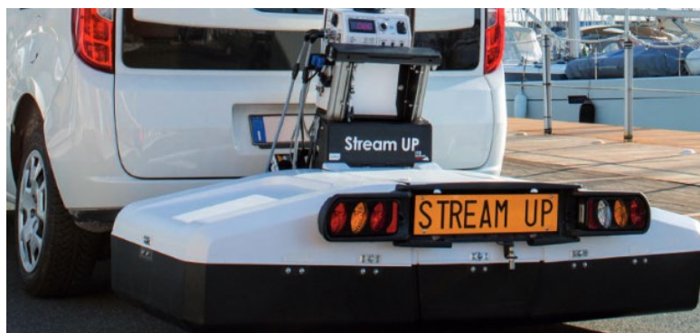
Figure 80. Stream UP System Mounted onto Survey Vehicle (idsgeoradar.com)
