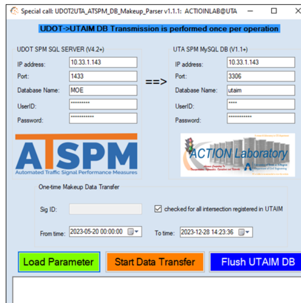
Figure 5-36: Transferring the ATSPM data from the UDOT-ATSPM database to the UTAIM database.
