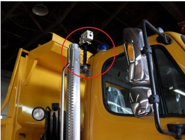
Figure 2-43 Two different winter operations vehicles with laser projection equipment installed on them (Laserline, 2018)
