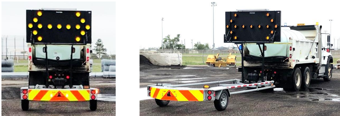
Figure 5-4 Recommended arrow board on the back of a winter operations vehicle (Amarillo District)
