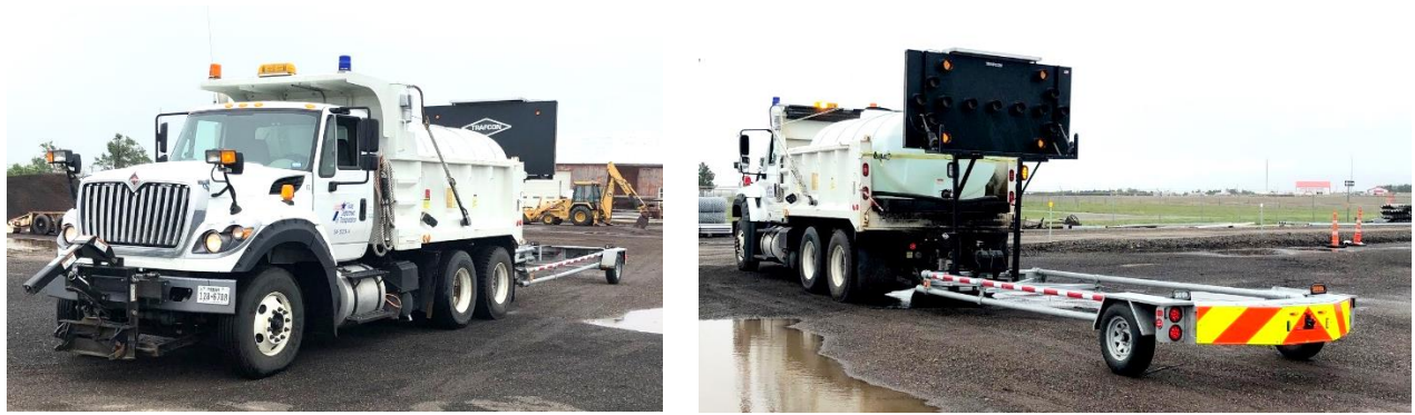
Figure 4-8 Front (left) and back (right) of winter operations vehicle attached to a TMA
