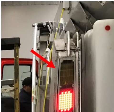
Figure 5-2 Recommended heated lens used with warning lights (Kansas)
