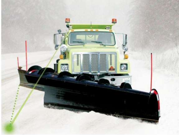
Figure 2-42 Laser path guidance system illustration and actual laser projection on the road from a winter operations vehicle (Laserline, 2018)
