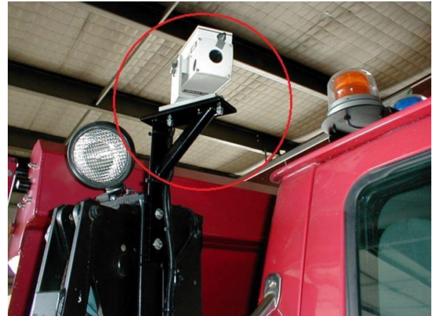
Figure 2-43 Two different winter operations vehicles with laser projection equipment installed on them (Laserline, 2018)
