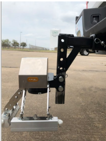
Figure 9: Scanner connected to the hitch of the pick-up truck.
