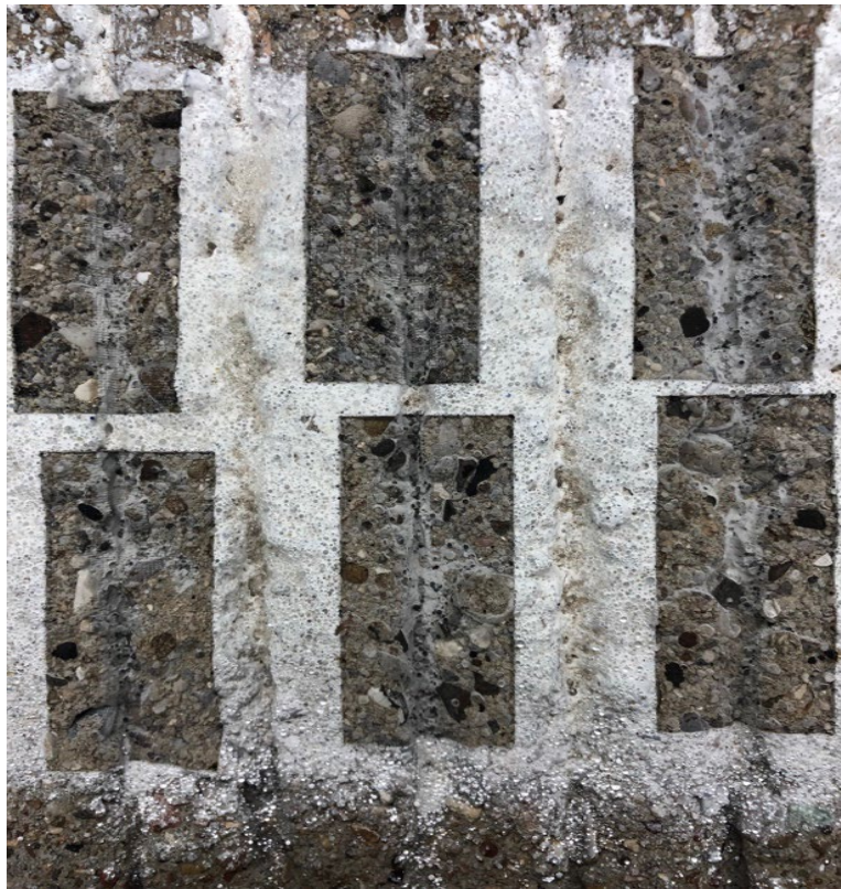
Figure 6: Photograph of a white paint stripe on concrete specimen with different ablated regions.
