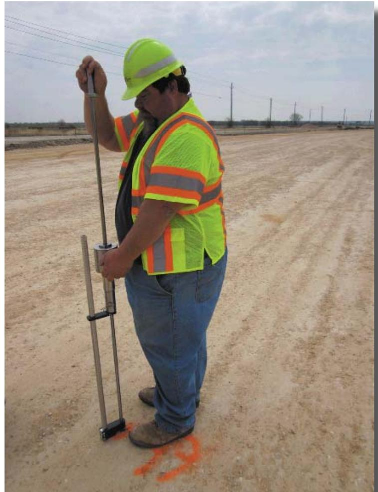
Figure 1. Testing for Penetration Index with Dynamic Cone Penetrometer.
