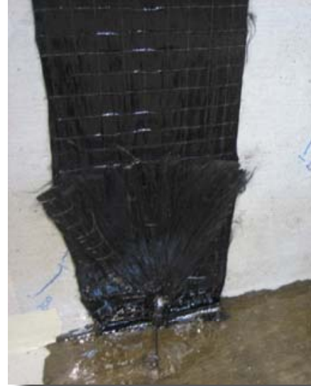
Figure 1: (a) Full-scale bridge I-girder strengthened using anchored CFRP (after testing); (b) CFRP anchor close-up
