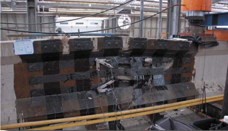
Figure 1: (a) Full-scale bridge I-girder strengthened using anchored CFRP (after testing); (b) CFRP anchor close-up
