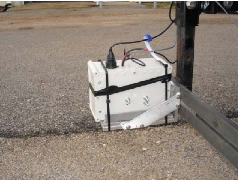
Prototype Profiler Module Mounted in Front of Test Vehicle.
