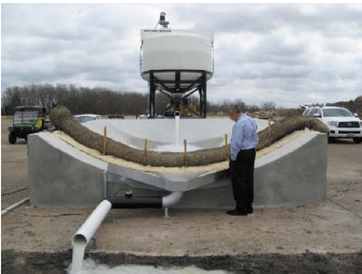
Figure 1. Sediment Retention Device Evaluation Flume.
