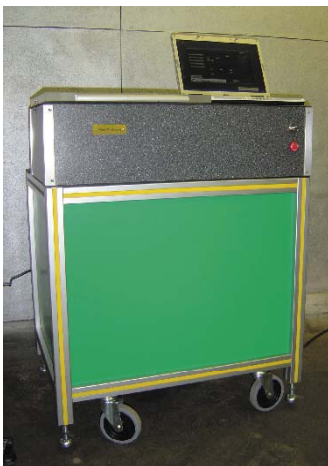
Overlay Tester-based Crack Sealant Adhesion Tester.
