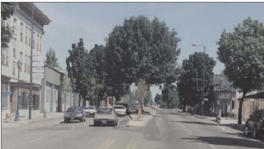
Figure 5. Martin Luther King Boulevard (State Highway 99) in Portland, Oregon, was a major state highway; it has been modified to four lanes with curb parking, landscaped median, and sidewalk landscaping in keeping with its new use as a local arterial.
