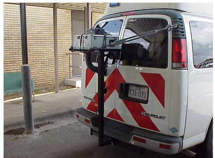
Figure 4. Scanning Laser System Mounted on TxDOT TMV
