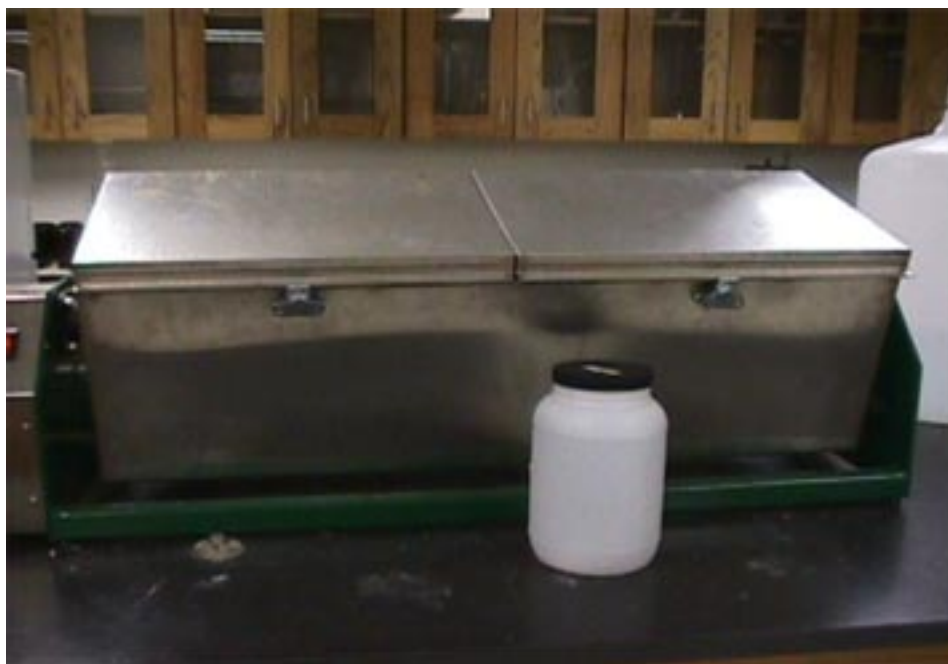
Figure 2: Extraction Vessel and Tumbler
