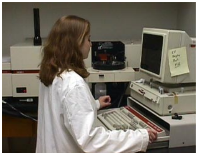
Figure 1. Graphite Furnace Atomic Absorption Spectrometer
