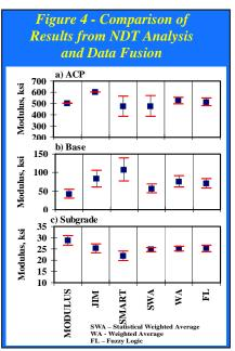
condition. This process has inherent nonuniqueness that can be minimized with input from more than one NDT device. The integration method, therefore, has a distinct advantage because it uses multiple sources to extract relevant pavement response to ensure that the properties specified are most representative of the pavement condition.
