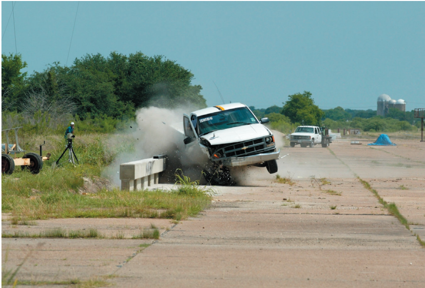
Vehicle during collision with 30-inch version of bridge rail.
