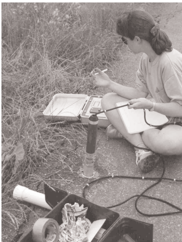
Figure 1. Probe being inserted into access tube
