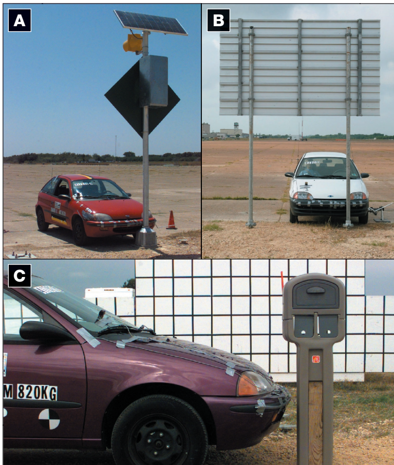
Figure 1. a) Tests in this project combined solar-powered units with flashing beacon assemblies; b) Properly installed dual slip-base sign supports serve as a safe, cost-effective system; c) In all three tests performed, molded plastic mailbox units satisfied evaluation criteria.
