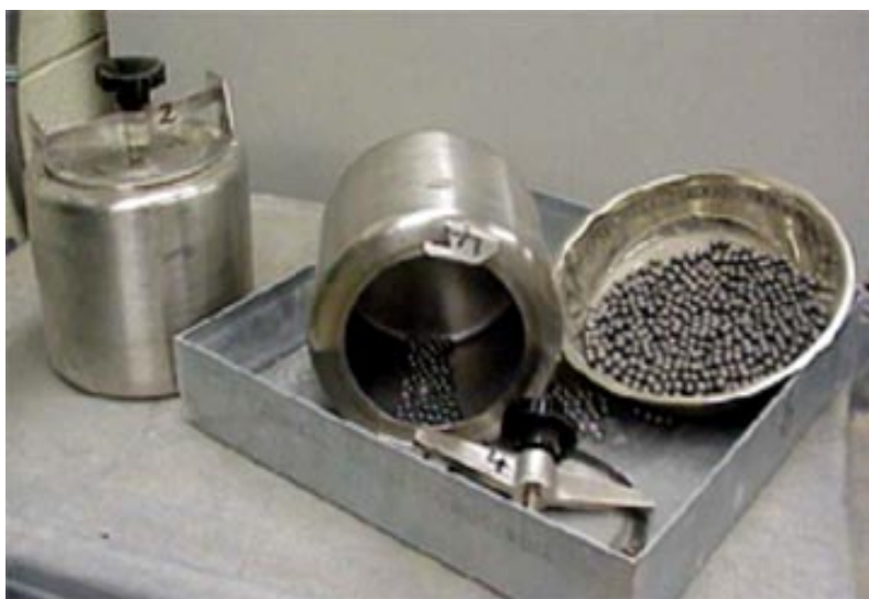
Figure 1. Steel jar and charge used in micro-deval test
