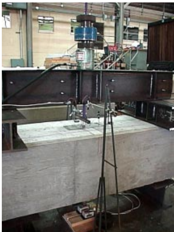
Figure 2 - Setup for Phase 1 Pullout Test
