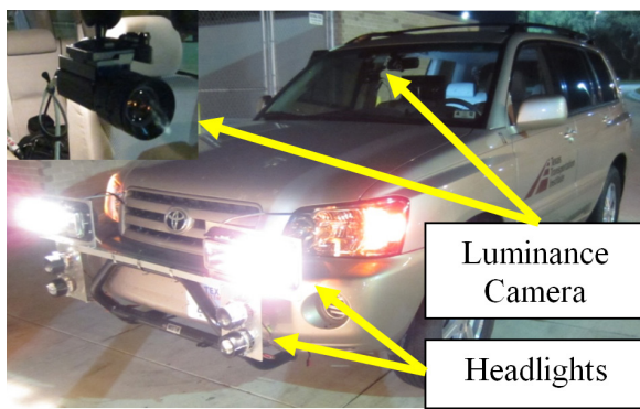
(a) Lighting and Luminance Camera Setup
