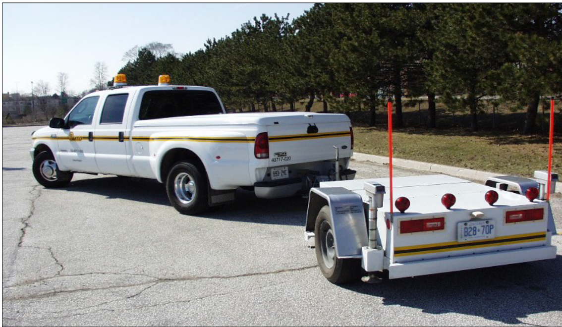
Figure 1. New ASTM E274 Skid Measurement System.
