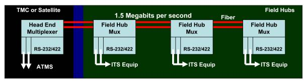
Figure 1. Traditional T1 Field Hub and Satellite Architecture.
