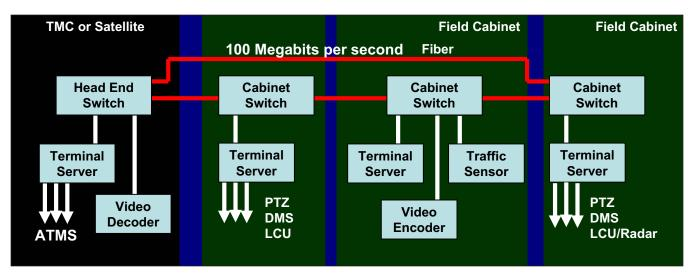
Figure 3. Ethernet Replacing T1.
