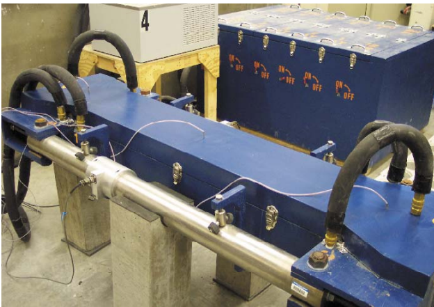
Figure 1: Cracking frame test set-up.
