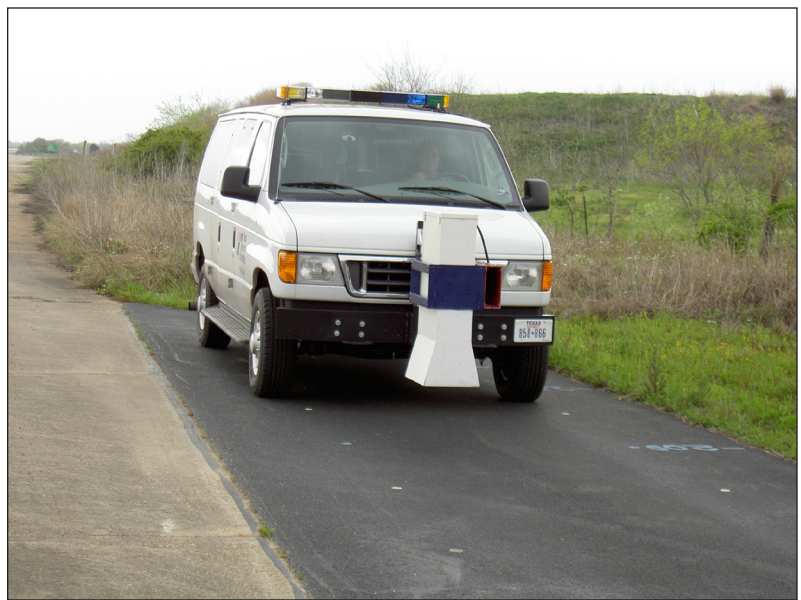
Figure 1. TxDOT's GPR System.
