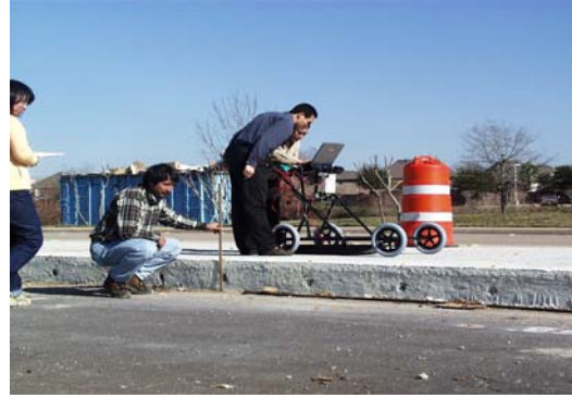
Figure 2. Field test of the developed thickness radar over new pavement with steel rebar (Picture taken by Ed Oshinsky).
