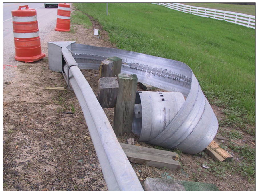
Figure 2. Photograph Taken during Pilot Test of an ET-2000 Single Guardrail Terminal That Performed as Intended.
