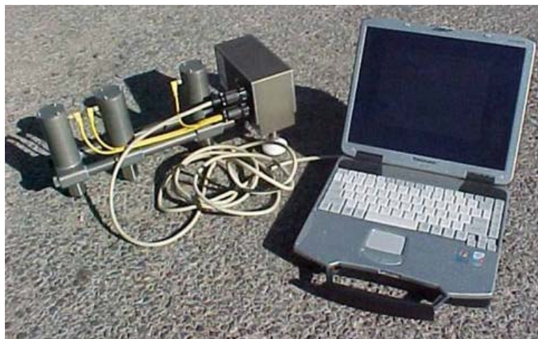
Figure 1 – Portable Seismic Pavement Analyzer
