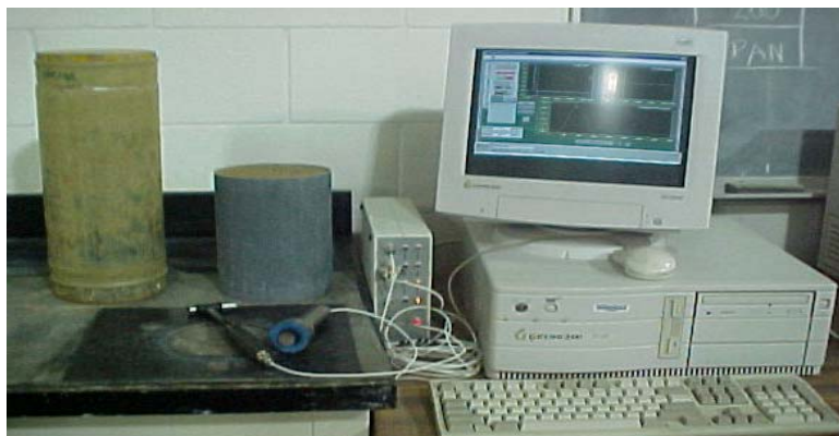
Figure 2 – Free-Free Resonant Column Device
