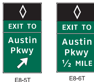
Figure 2G-11. Examples of Barrier-Mounted Guide Signs for an Intermediate Egress from Preferential Lanes
