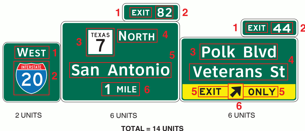
Figure 2E-1T Example of Guide Sign Information Units
