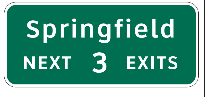
Figure 2E-33. NEXT EXITS Sign
