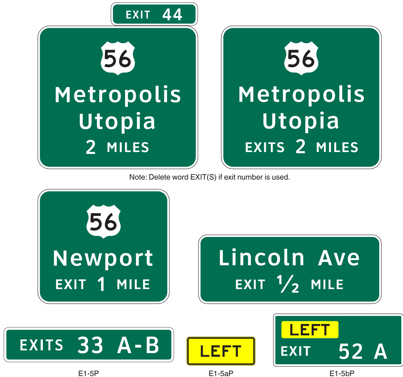
Figure 2E-22. Examples of Interchange Advance Guide Signs, Exit Number Plaques, and LEFT Plaque
