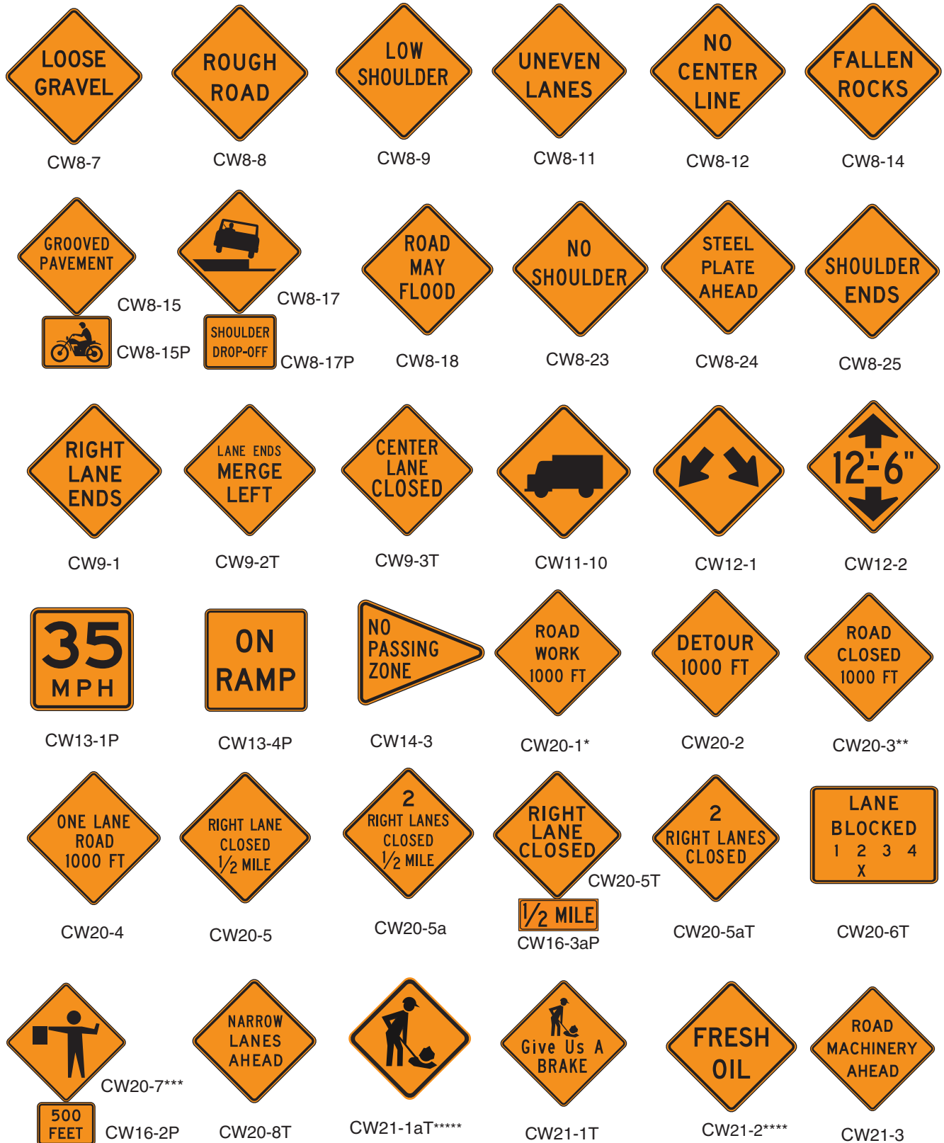
Figure 6F-4. Warning Signs and Plaques in Temporary Traffic Control Zones (Sheet 2 of 3)
