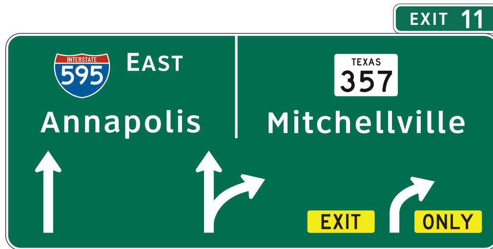
Figure 2E-3. Overhead Arrow-per-Lane Guide Sign for a Multi-Lane Exit with an Option Lane
