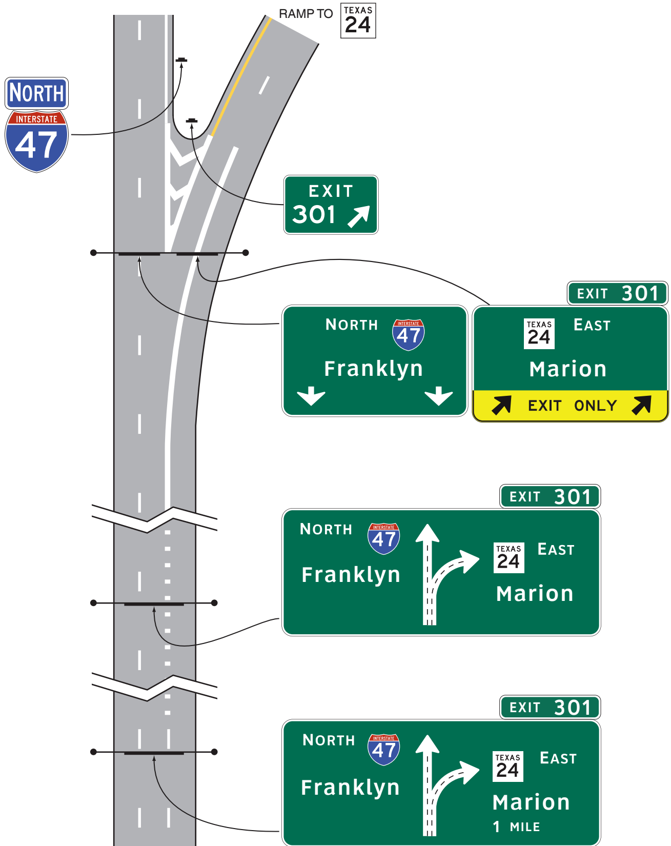
Figure 2E-8. Diagrammatic Guide Signs for a Two-Lane Exit to the Right with an Option Lane
