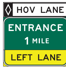
Figure 2G-5. Example of an Overhead Advance Guide Sign for a Preferential Lane Entrance
