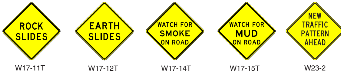
Figure 2C-6. Roadway and Weather Condition and Advance Traffic Control Signs and Plaques (2 of 2)
