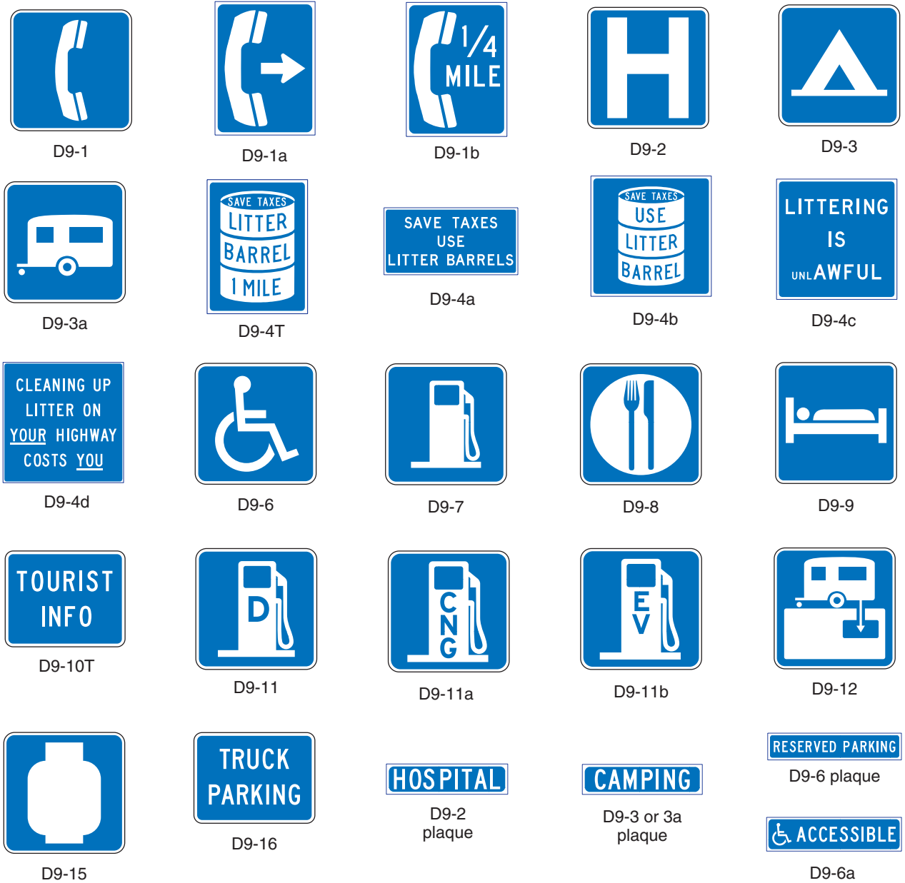
Figure 2D-11. General Service Signs
