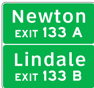
Figure 2E-17. Supplemental Guide Signs for Multi-exit Interchanges
