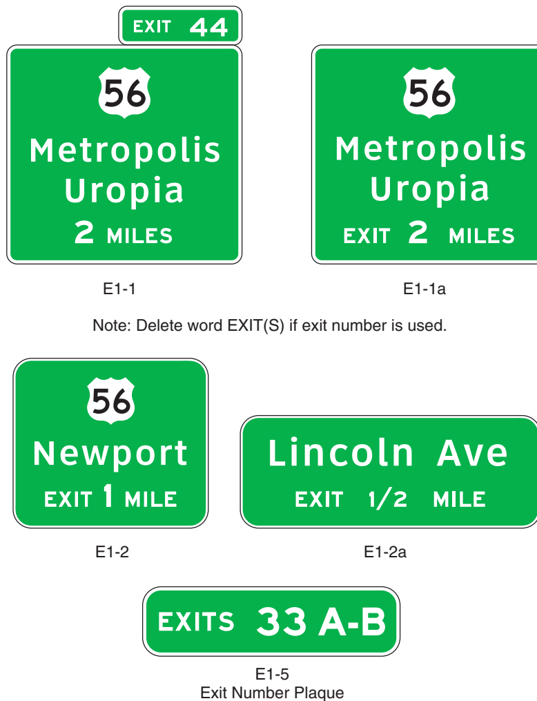
Figure 2E-15. Examples of Interchange Advance Guide Signs
