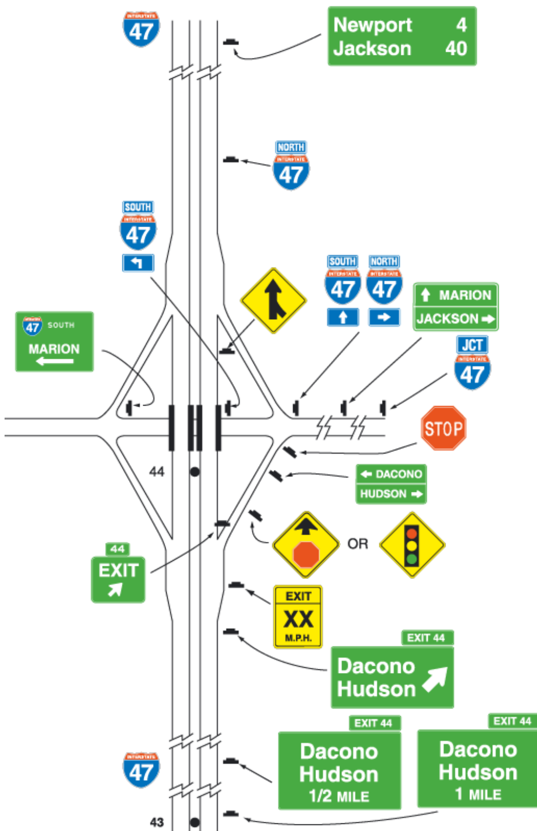
Figure 2E-28. Typical Diamond Interchange Guide Signs
