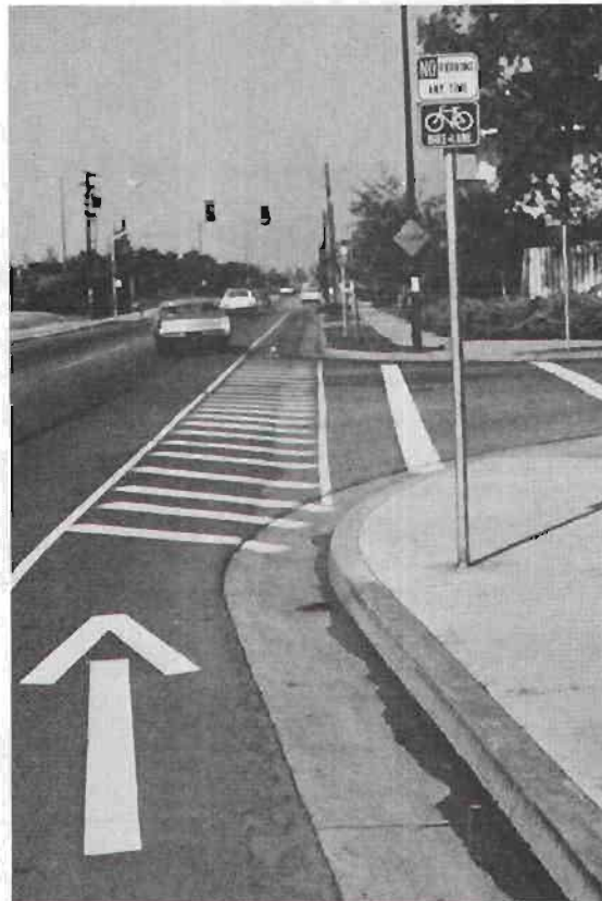
Bikeway Marked Thru Intersection With Diagonal Lines For Added Visibility And Emphasis
