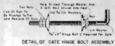
DETAIL OF GATE HINGE BOLT ASSEMBLY
