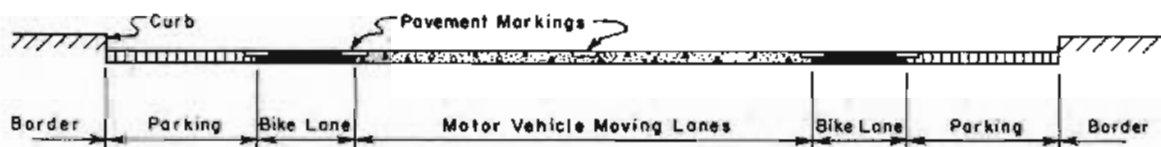
(b) Parking permitted - Bicycle lane located between parking lane and motor vehicle moving lanes
