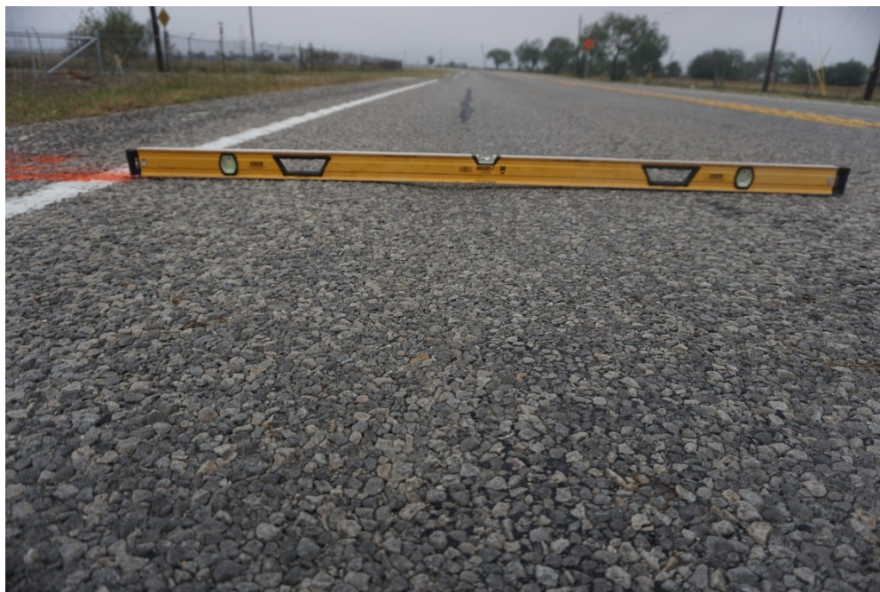
Figure 63. Picture of Pavement Rutting on SH 202.
