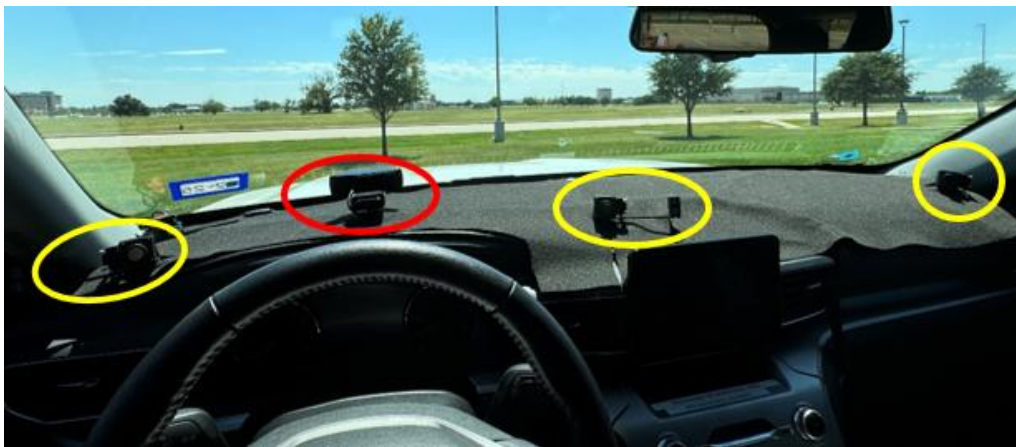
Figure 11. Smart Eye Camera Setup on Vehicle Dashboard.
