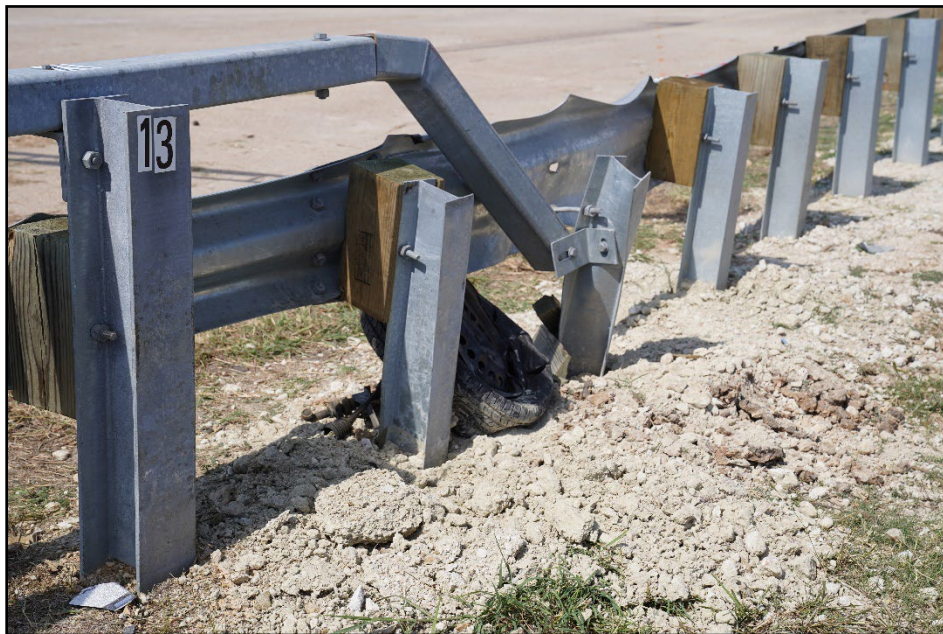
Figure 6.6. Transition after Test from the Field Side of the Installation for Test 441203-01-1.
