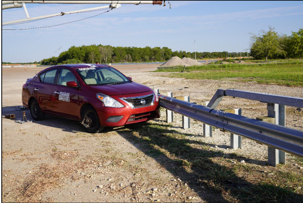
Figure 6.1. Transition and Test Vehicle Geometrics for Test 441203-01-1.
