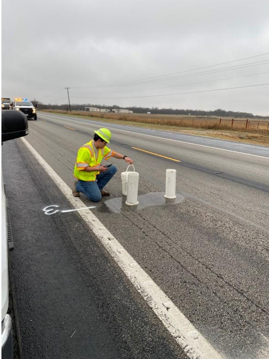
Figure 71. Water flow testing.
