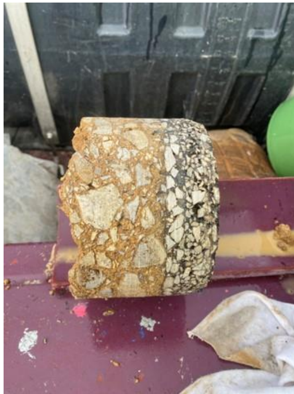
Figure 74. Close-up of US 183 PFC core.
