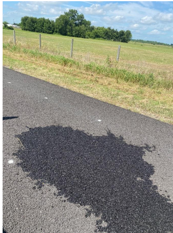
Figure 92. Water poured onto the PFC surface.
