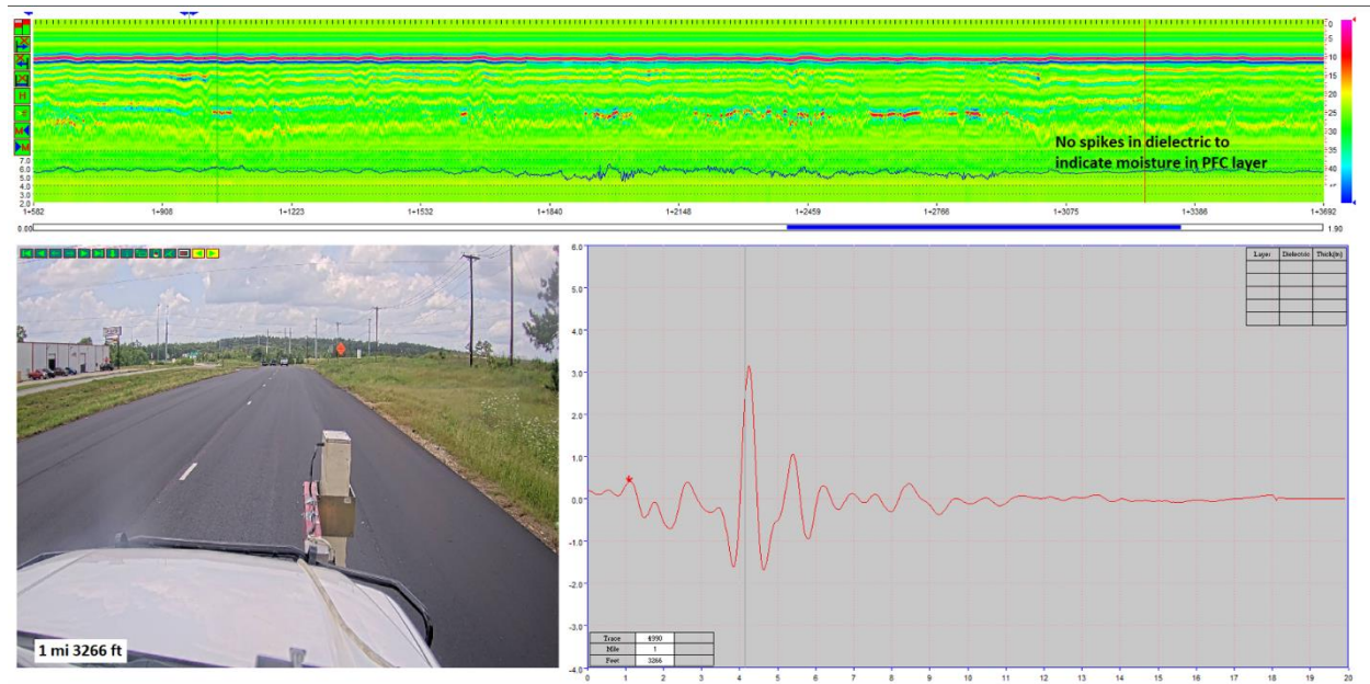
Figure 109. GPR taken 1 week after construction showing overall satisfactory performance and no trapped moisture.
