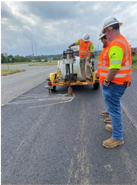
Figure 105. Coring operation over bulged pavement area: (a) coring rig, and (b) cores taken showing the new overlay bonded to the old PFC.
