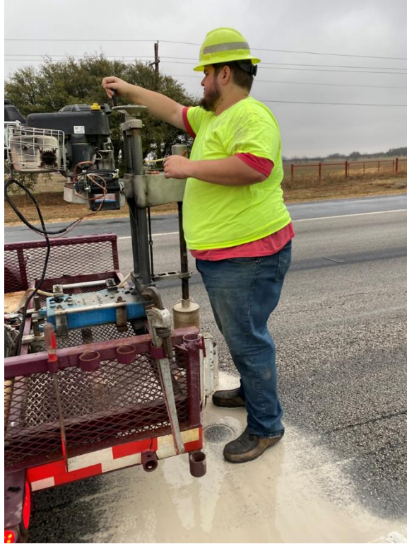
Figure 73. Coring of fine PFC.
