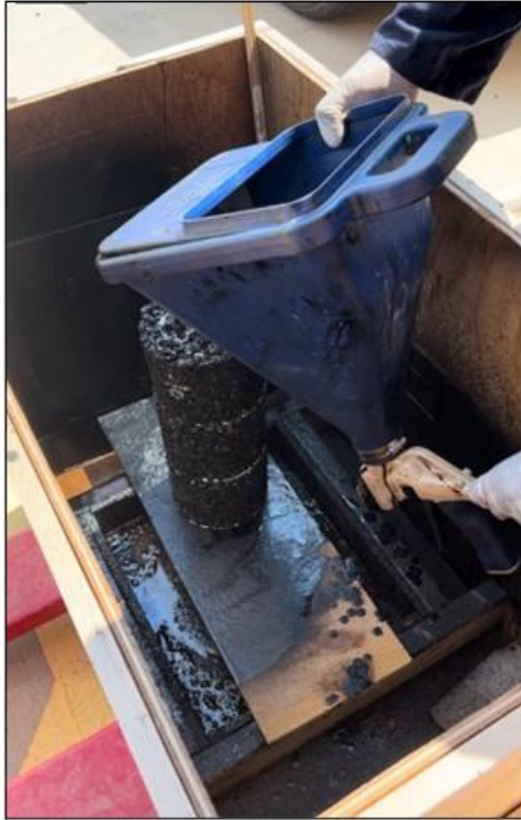
Figure 80. Cantabro specimens stacked rejuvenator application.
