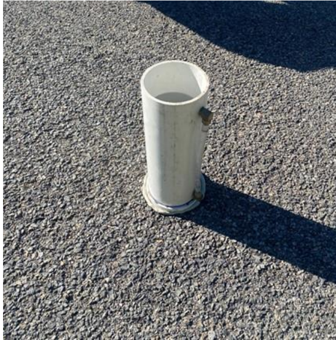
Figure 56. No water flowing in old PFC.
