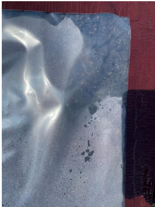
Figure 94. Moisture condensation on the underside of the plastic.
