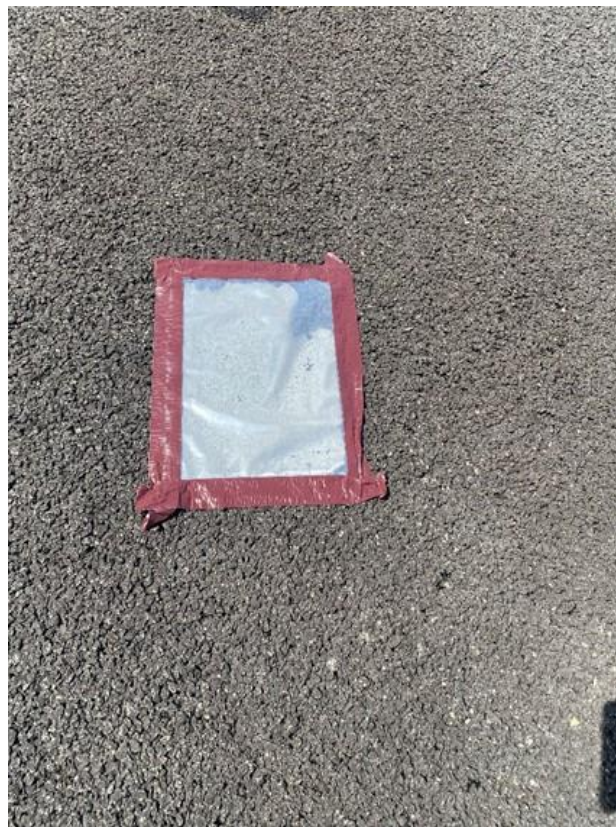
Figure 10. Moisture test on PFC pavement surface.
