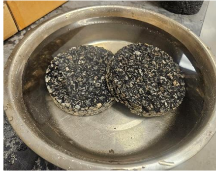
Figure 87. Lufkin cores being saturated under water.
