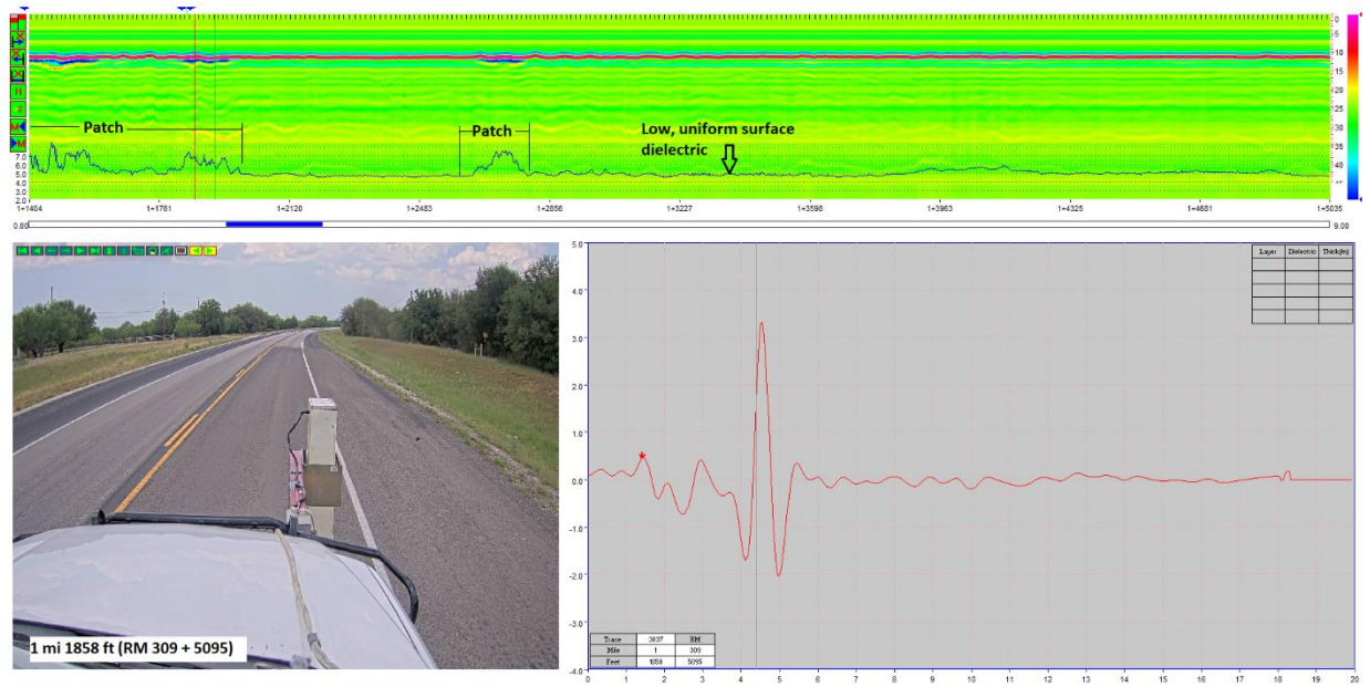
Figure 69. GPR data on US 183 south of Breckenridge.
