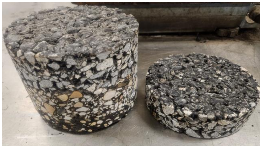
Figure 86. Lufkin core before and after saw cut.
