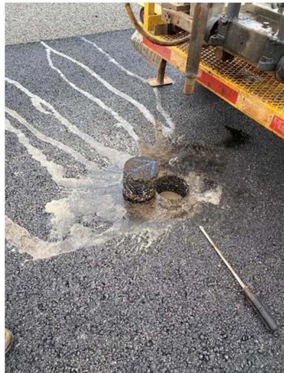
Figure 105. Coring operation over bulged pavement area: (a) coring rig, and (b) cores taken showing the new overlay bonded to the old PFC.
