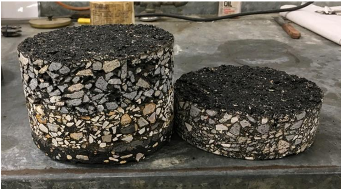
Figure 106. Photo of core after shear test.
