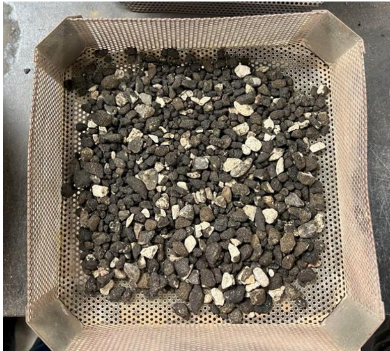
Figure 76. RAP sample after the ignition oven.
