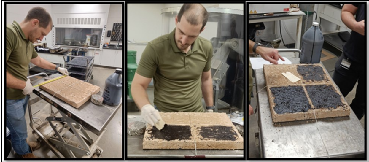
Figure 29. Priming of Slabs in Four Quadrants.
