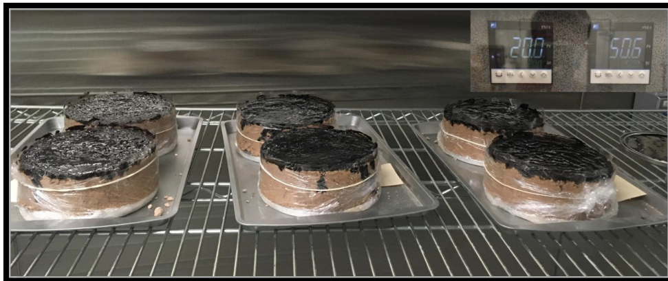
Figure 13. Specimens in the Test Environmental Condition (20°C and 50% RH).
