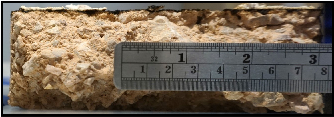
Figure 16. Example of Prime Penetration Depth in the Flexible Base.
