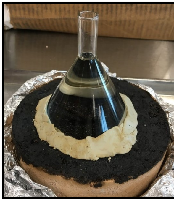
Figure 10. Modified Ring Test with Plumber's Putty.
