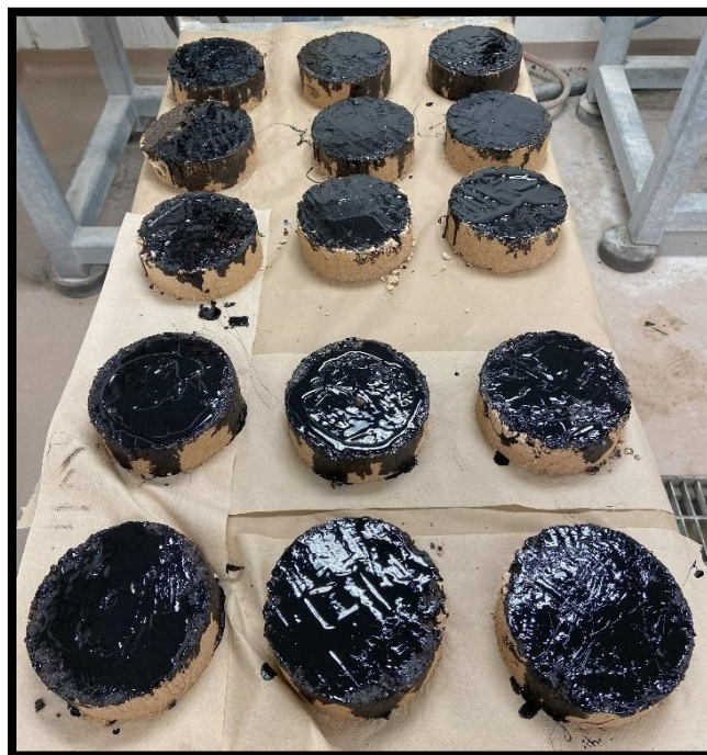
Figure 19. Primed Specimens with Asphalt Surfacing.
