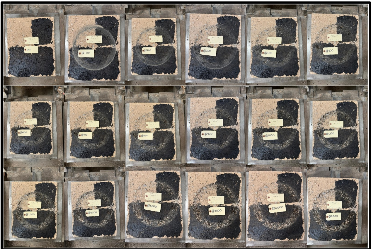
Figure 31. Three-Wheel Polisher Test of Slabs at Various Stages.
