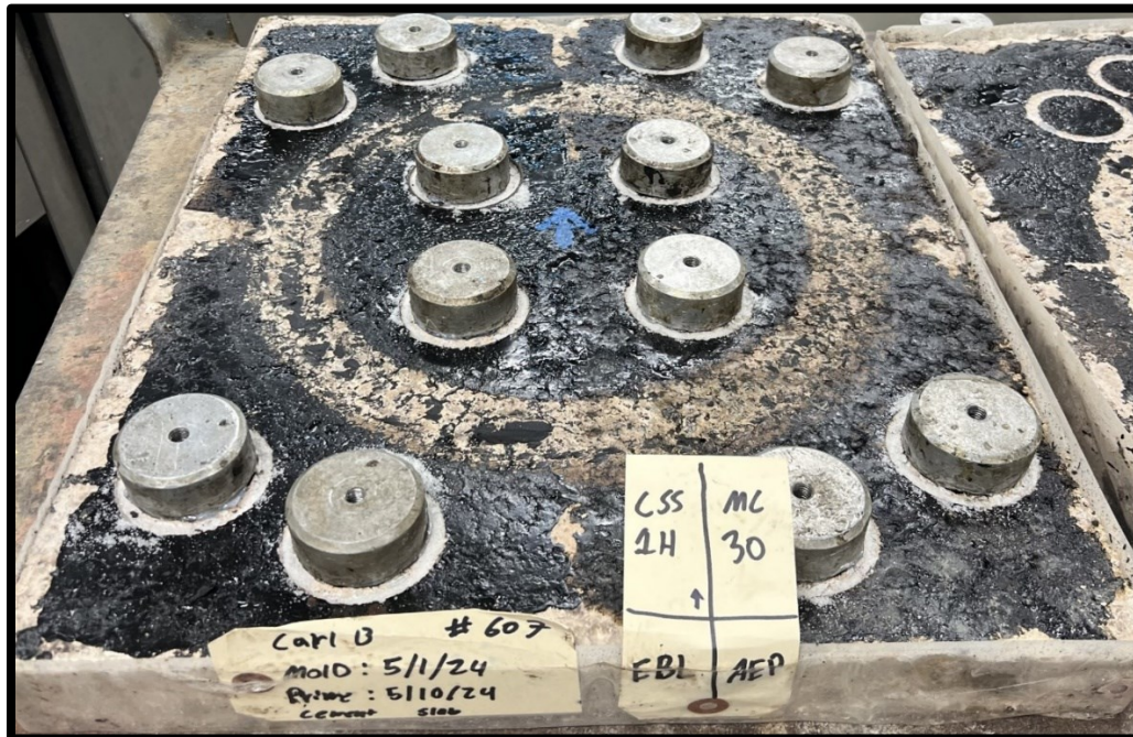
Figure 25. Torque Test Locations on Cemented Slabs.
