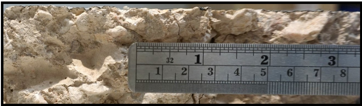
Figure 17. Example of Prime Penetration Depth in the Cement-Treated Base.
