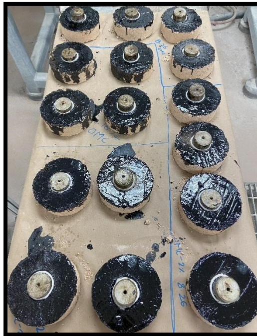
Figure 20. Pucks Glued to Asphalt Surfacing.
