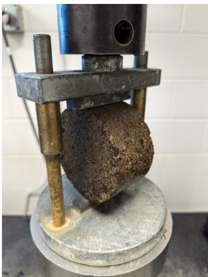
Figure 1. 4-Inch-Diameter Soil Specimen Tested for Indirect Tensile Strength.
