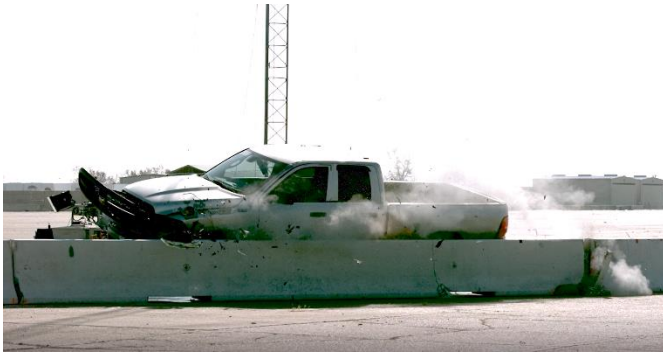
Figure 1. Full-Scale Test on Damaged PCB.
