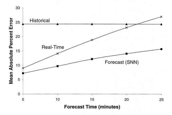
Figure 1: MAPE versus Forecast Travel Time for U.S. 290 Link during the AM Peak Period
