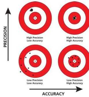
**Figure 3.11 Dartboards Showing Different Accuracy and Precision Scenarios**
