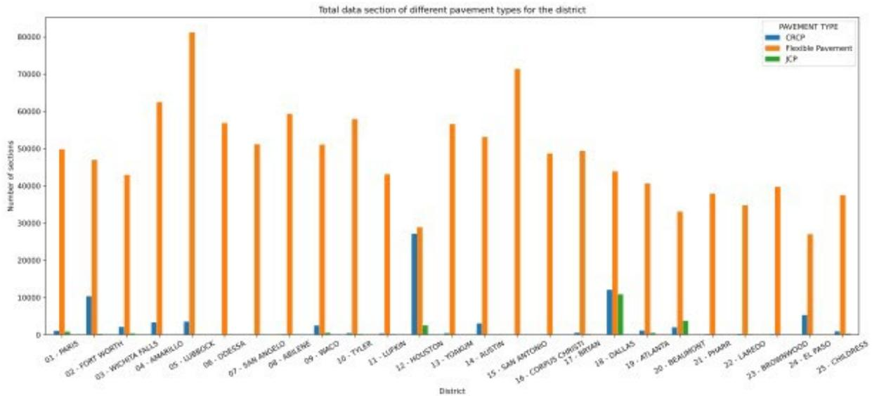
**Figure 3.4 Data Collection Sections of Pavement Types For 25 Districts**
