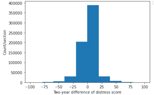
**Figure 3.14 Tolerance: Two Years' Distress Score within 15 points (2014-2020)**
