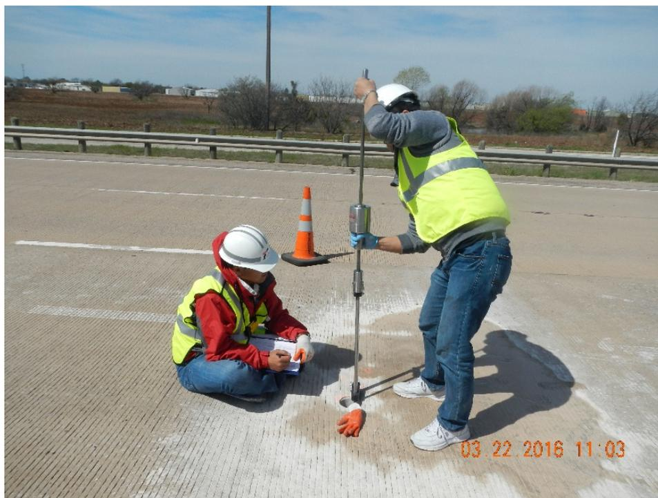
**Figure 3.20 DCP testing on US 281**
