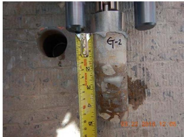
f. Failure mode determination
