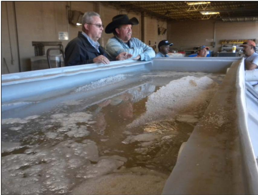
**FIG 5.** The TxDOT Childress District invested in a salt brine manufacturing system to make their own homemade salt brine
