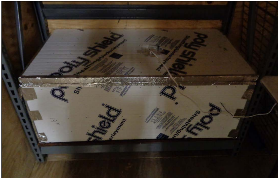
Figure 7.2 Photograph of freezing box inside cold box.
