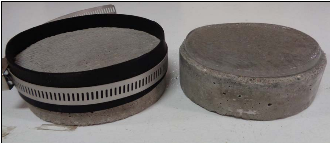
Figure 7.4 Photograph of mortar specimens for disbondment testing, with and without ice.
