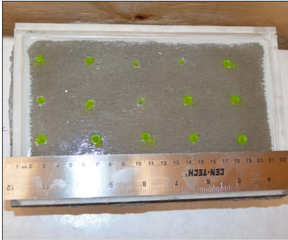
Figure 7.3 Photograph of mortar specimen immediately after addition of salt solution.
