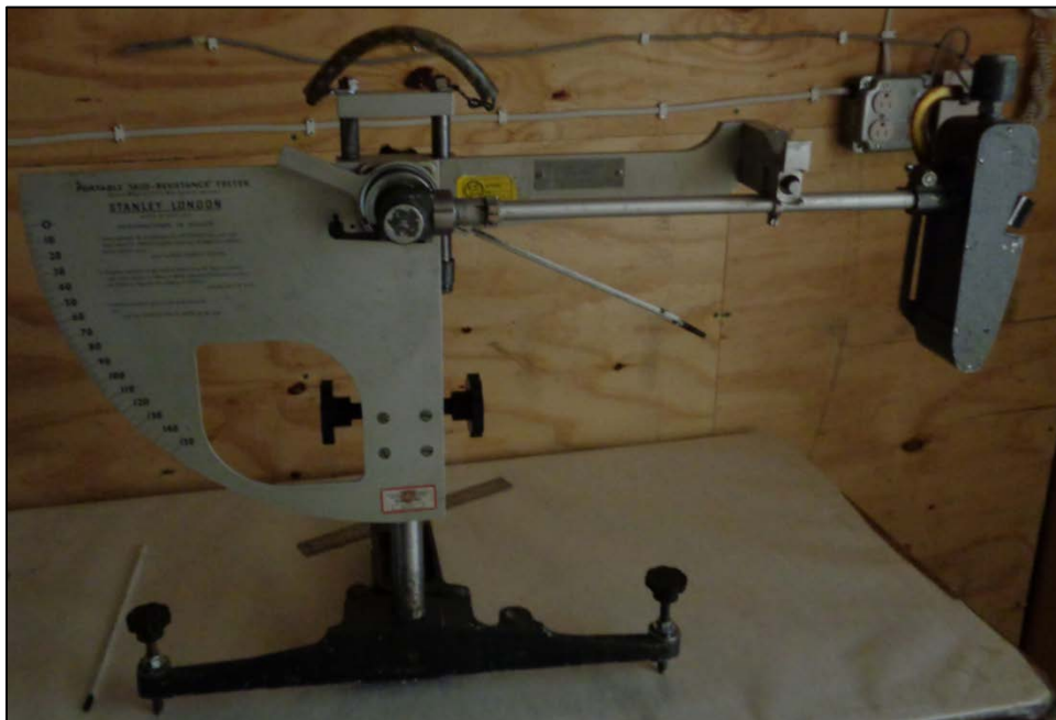
Figure 7.6 British Pendulum Skid Resistance Tester used for friction testing.
