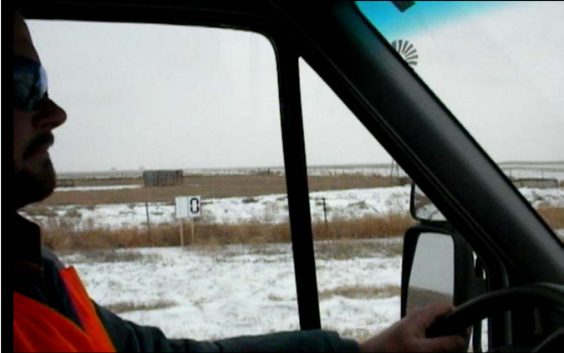
Figure 3.8. Images were taken at 200-ft intervals as delineated in each test section (station marker in background)
