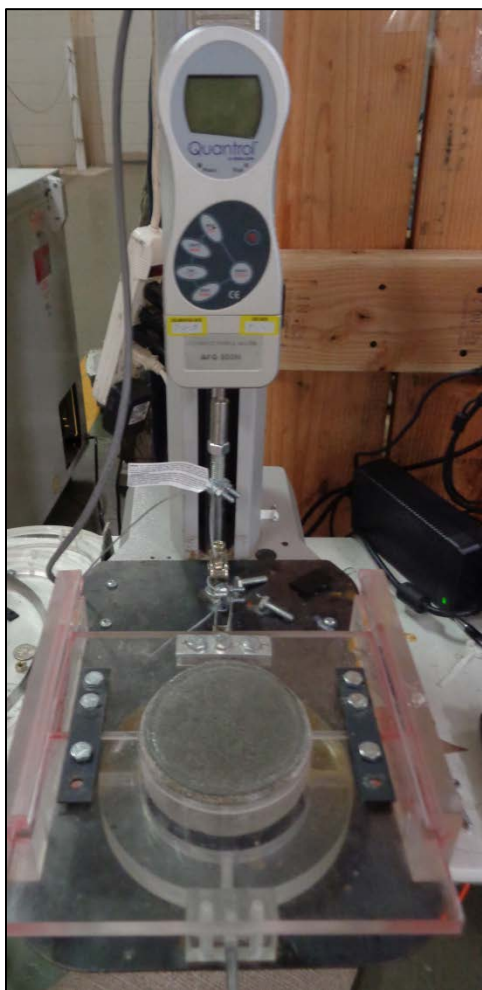
Figure 7.5 Mecmesin MultiTest 1-d motorized test stand used for disbondment testing.
