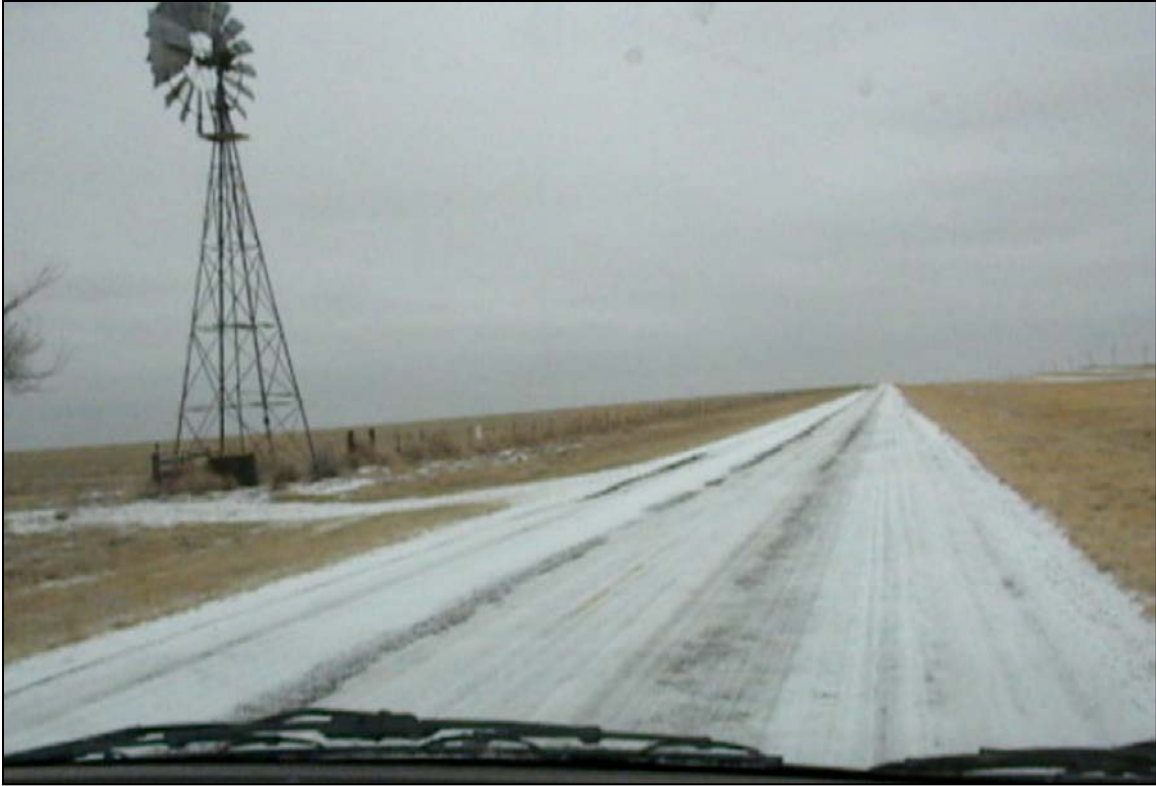
Figure 4.6. Road Surface Condition Before Plowing, Drive Lane Treated w/Road Salt/ Opposite Lane Control
