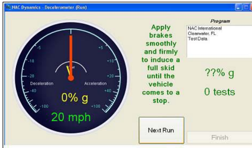
Figure 3.15. Apply Brake Test Run Prompt, NAC Dynamic Friction Decelerometer
