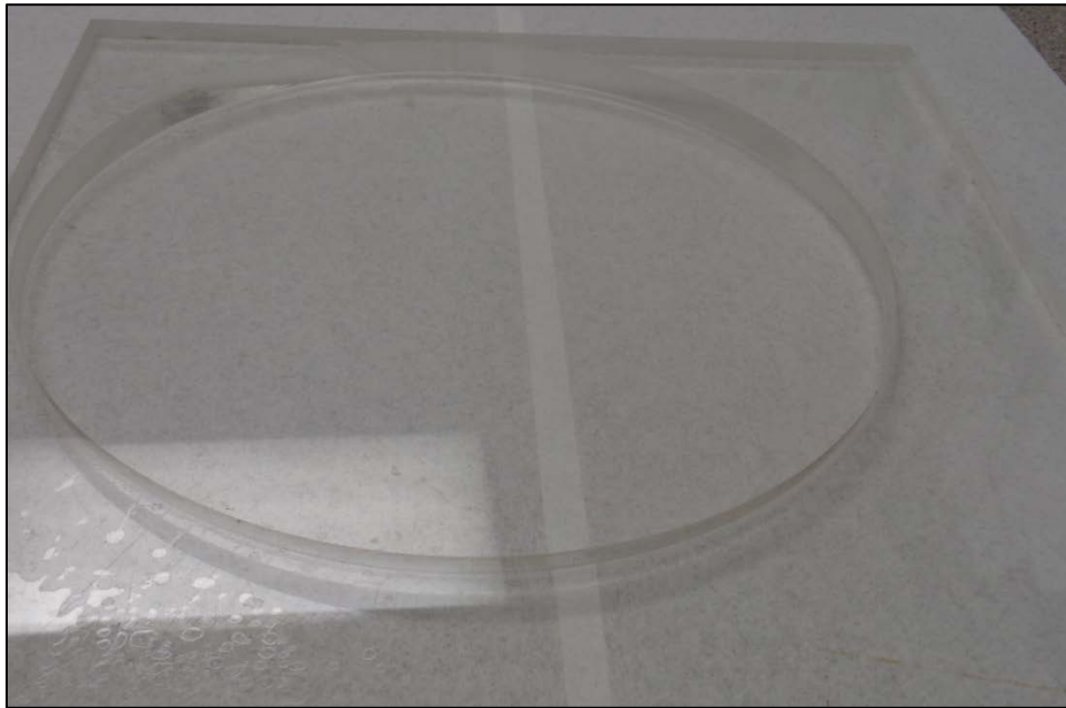
Figure 7.1 Circular acrylic dish used for ice melting.
