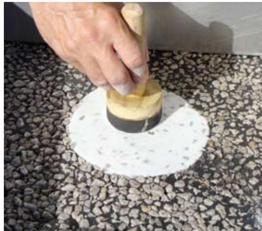
Figure 9. Measuring Four Diameters of the Resulting Circle for Averaging.
