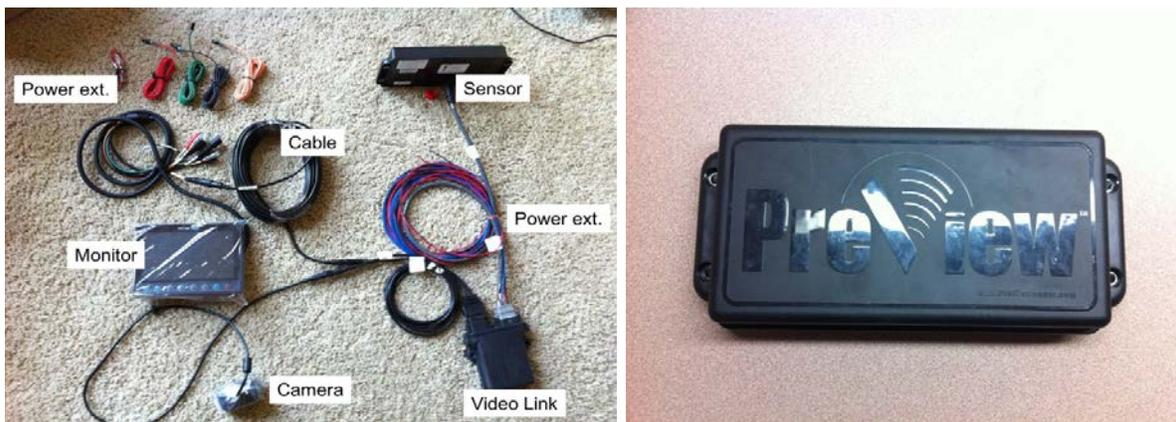
**Figure 5.2 WorkZone: Major Component (Left) and a Pulsed Radar Sensor (Right)**
