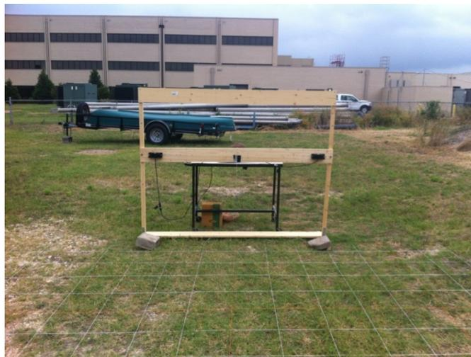
Figure 5.10 Frame and Measurement Grid Setup for Static Tests
