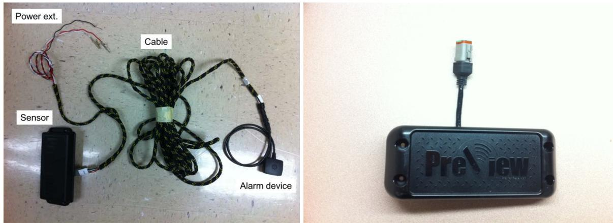
**Figure 5.4 WorkSight: Major Component (Left) and a Pulsed Radar Sensor (Right)**
