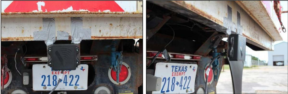
Figure 5.9 “L” Shape Bracket to Hang on the Sensor
