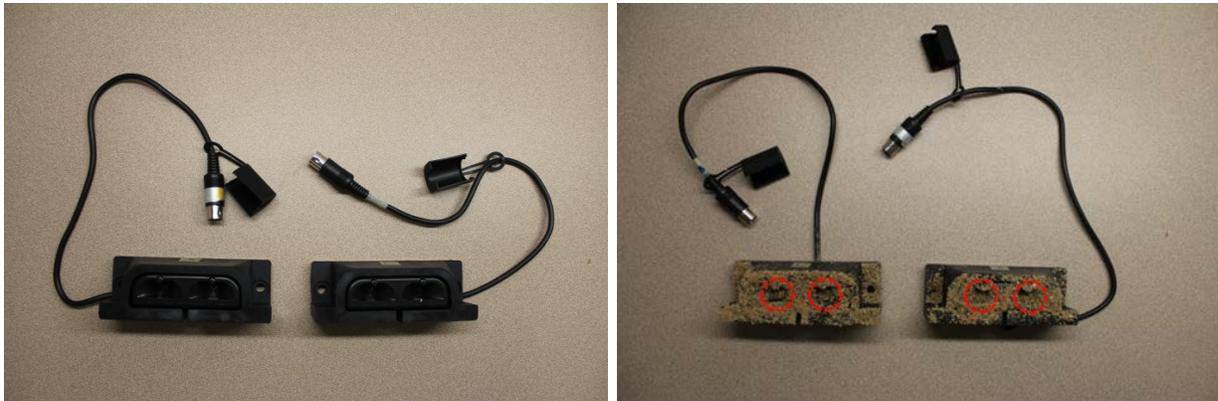
**Figure 5.26 HCS-700 System: Before and After Soil Coverage**
