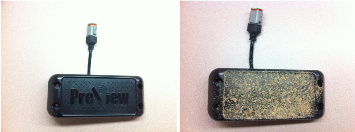
**Figure 5.27 WorkSight System: Before and After Soil Coverage**
